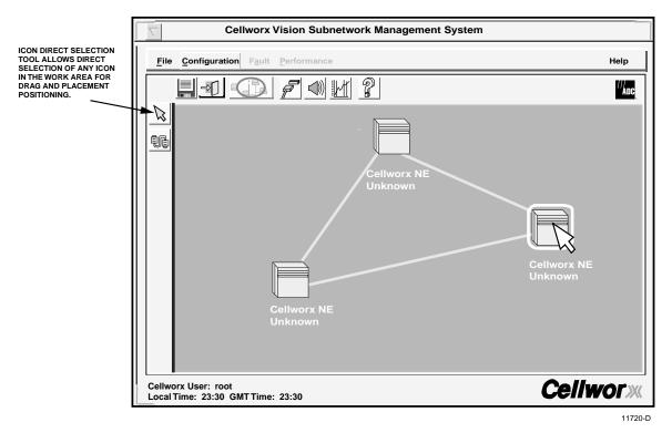
Figure 740-5. Cellworx Vision Redrawing ICON Layout
